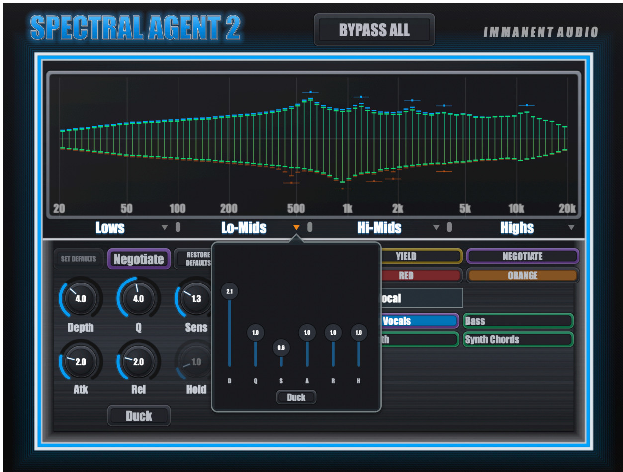
The Lo-Mids band panel. D, Q, S, A, R and H multiply the pair's Depth, Q, Sens, Atk, Rel and Hold in that band, and Duck routes that band on its own. The arrow above turns orange once a band has been moved off its defaults.
